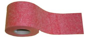
Warmup's 3-ply waterproof membrane products protect floors and walls under thin-set tile installations from substrate cracks and moisture migration. It is comprised of 2 outer polypropylene layers and one inner polyethylene waterproofing membrane and exceeds testing requirements per ASTM 118.10. The range is comprised of a 35ft roll of 5"-wide membrane, along with outer corners and inside corners.
