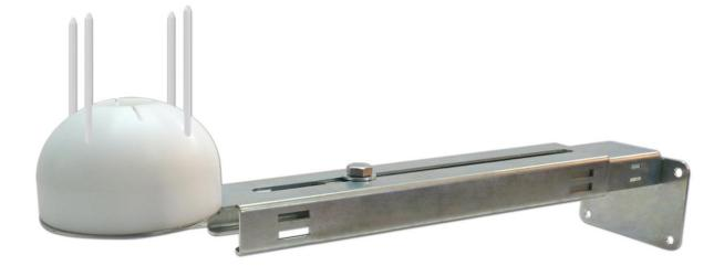
The AIRSENSE/19 is connected to the Snow Melting Controller (PYROCON19) with a 30 feet (10 m.), 24V 4 wires cable and communicating with the controller, providing the temperature value and the snow detection based on the adjustable parameters.
