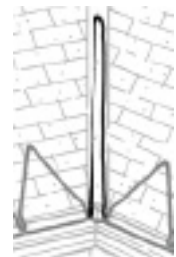
Figure 4: Cable pattern in valley
