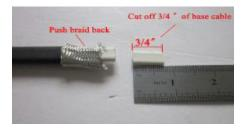
To prevent short circuits, do not connect the bus wires together. Keep braid out of heat shrink cap.
