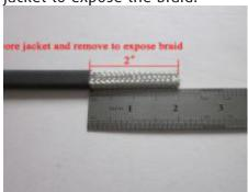
**CAUTION:** When removing the outer jacket, be careful not to damage the braid or the base cable insulation.
