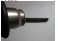
**8.** While the shrink tubing is still hot, gently squeeze the end of the shrink tube with pliers and hold until cool. The end must remain visibly sealed when the pliers are removed. If the tube does not remain sealed, then repeat steps 7 and 8.
