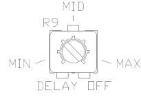
The DEL configuration switch activates the Delay-Off drying cycle timer on the DS- 9C. The timer allows the DS-9C to continue to operate and dry the heated surface through evaporation once precipitation has stopped. The drying cycle reduces the chance of moisture left behind refreezing into ice. This timer is restarted by each sensor trigger. Therefore, the DS-9C will MAX continue to operate as long as it is triggered, then for the Delay-Off period once the trigger clears.
