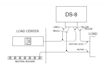
120VAC In, 120VAC Load, Heat Cable or Similar (Strap DS-8 for 120VAC Power)
