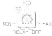
The DEL configuration switch activates the Delay-Off drying cycle timer on the DS- 8C. The timer allows the DS-8C to continue to operate and dry the heated surface through evaporation once precipitation has stopped. The drying cycle reduces the chance of moisture left behind refreezing into ice. This timer is restarted by each sensor trigger. Therefore, the DS-8C will continue to operate as long as it is triggered, then for the Delay-Off period once the trigger clears.
