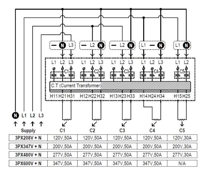
Note: Contactors 1,2,3 and 4 can be connected to any combination of 1 or 3 (triangle transform) heaters with and without Neutral.
