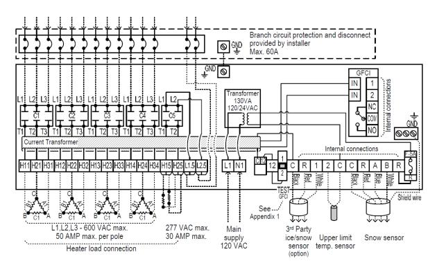
IMPORTANT: If the heaters are connected in stars, the neutral must pass through the internal current transformer ring and the external branch circuit protection.
