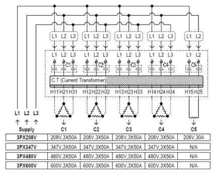
Note: Contactors 1 and 2 can be connected to any combination of 1 or 3 (triangle transform) heaters. Example: Contactor C1 can be connected to 3 heaters (triangle transform) and contactor C2 can be connected to 1 heater.
