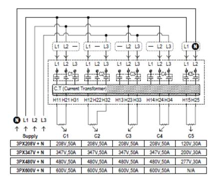
Option 2: 3 heaters per contactors C1, C2, C3 and C4 (triangle transform) and 1 heater per contactor C5
