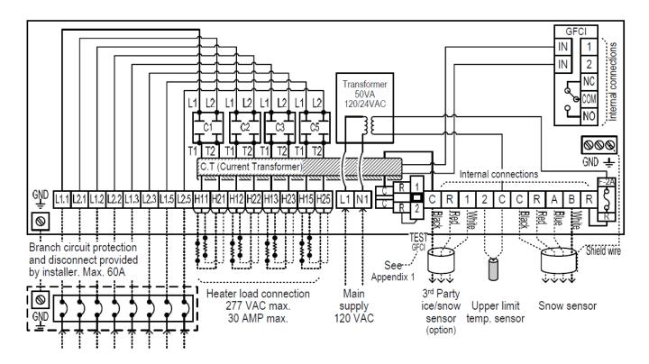
IMPORTANT: If the heaters are connected in stars, the neutral must pass through the internal current transformer ring and the external branch circuit protection.
