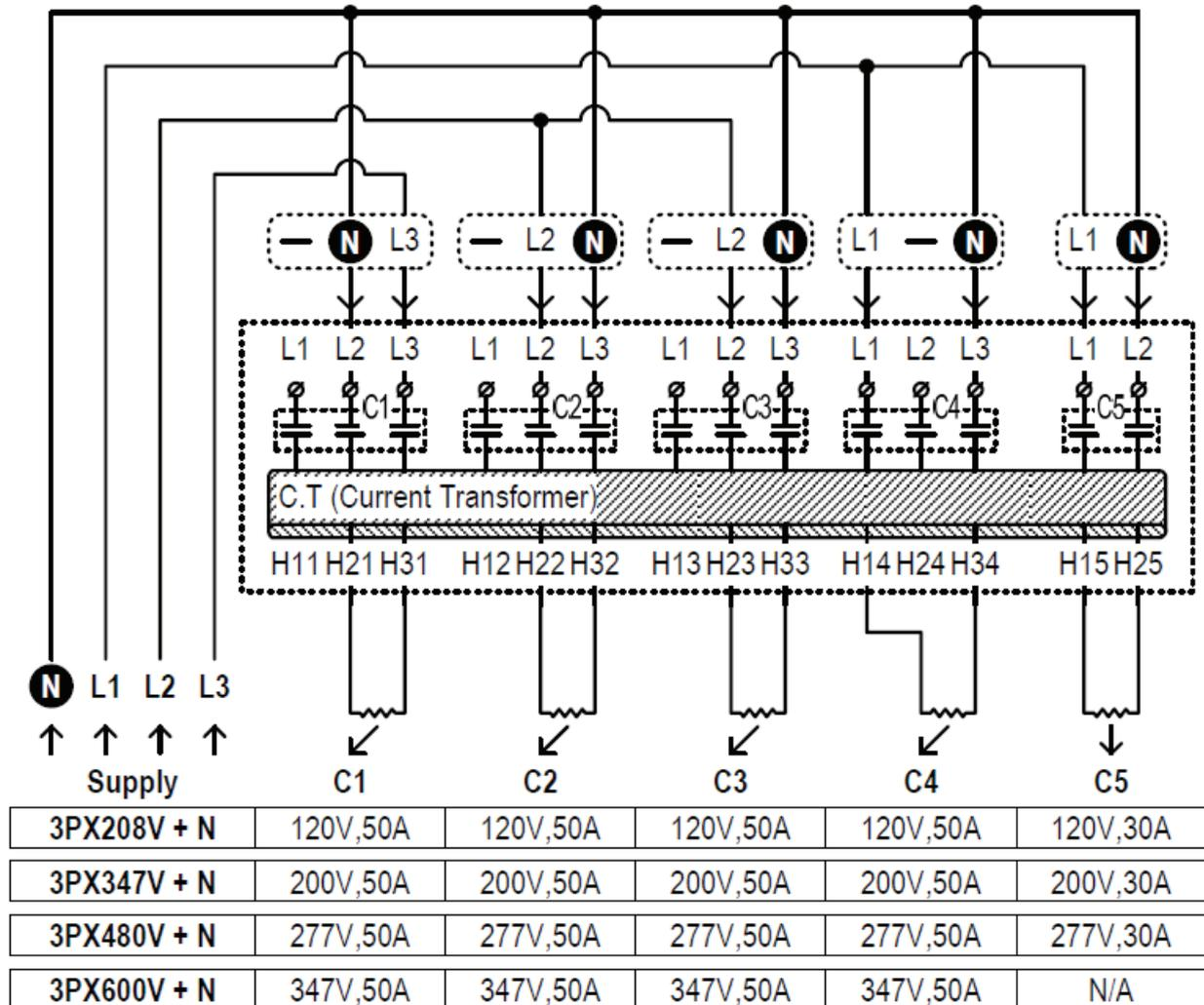
Note: Contactors 1,2,3 and 4 can be connected to any combination of 1 or 3 (triangle transform) heaters with and without Neutral.
