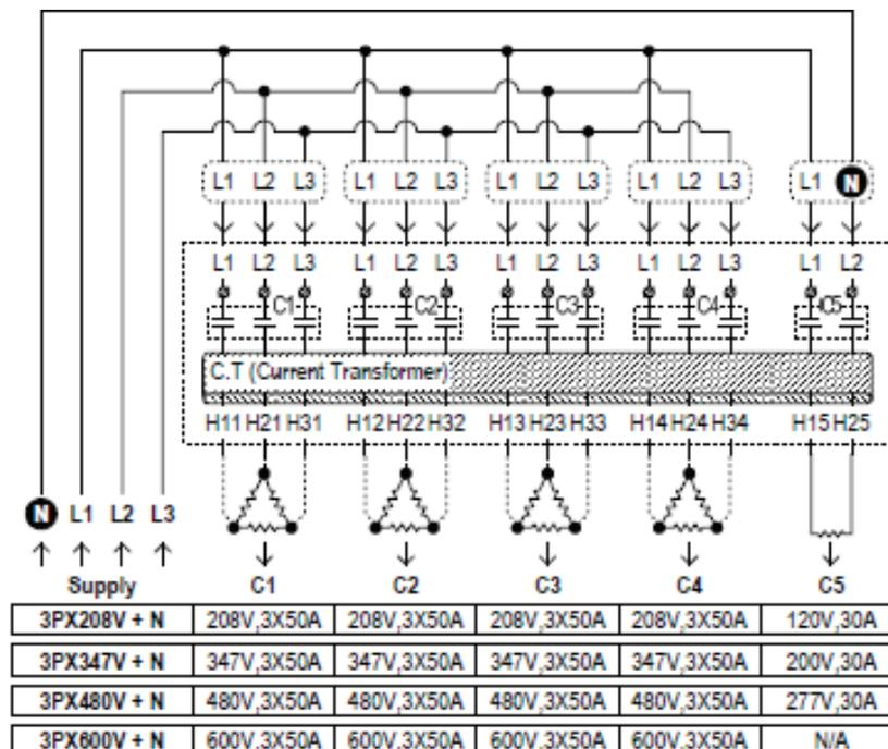
Option 3: 1 heater per contactors C1, C2, C3 and C4 and C5 (Neutral connected to C1, C2, C3, C4 and C5)
