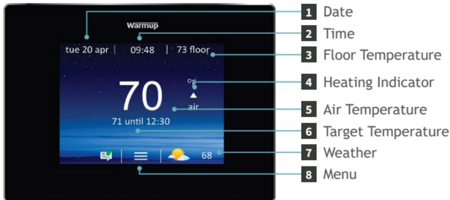
Once setup has been completed the thermostat will display the home screen. If you do not press any button for 1 minute the 4iE screen will dim and go into standby. To wake the 4iE just tap the screen or press the lock icon.
