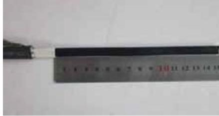
6. Cut PTC material to expose wires with utility knife. **Do not cut bus wires!**
