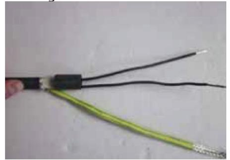
**13.** Heat the tube evenly until it shrinks and adhesive flows out of both ends.
