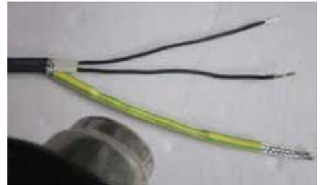
12. Slide "black shrinkable tube" of 1" (25mm) on the end of heating cable.
