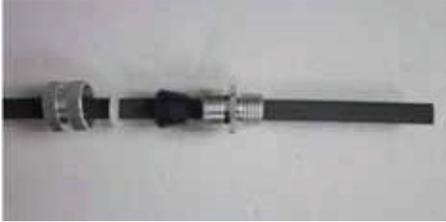
2. Slice completely around heating cable outer jacket, at a distance of 7" (178mm) from the end. Be careful not to cut braid or inner jacket. Then, bend the heating cable to break jacket where sliced, and peel off outer jacket.
