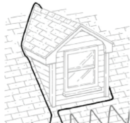
FIGURE 5: Cable pattern around a dormer
