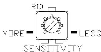
The DS-2C precipitation sensor is very sensitive and can detect a single snow flake or rain drop. However, if the DS-2C is mounted in an area susceptible to high winds, overhanging trees, or blowing ground snow, nuisance triggering may occur. While proper placement is the best remedy, the SENSITIVITY control can also be used to reduce nuisance triggering. An internal timer checks the precipitation sensor for moisture and compares cleared time with triggered time.
