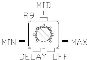
The DEL configuration switch activates the Delay-Off drying cycle timer on the DS-2C. The timer allows the DS-2C to continue to operate and dry the heated surface through evaporation once precipitation has stopped. The drying cycle reduces the chance of moisture left behind refreezing into ice. This timer is restarted by each sensor trigger. Therefore, the DS-2C will continue to operate as long as it is triggered, then for the Delay-Off period once the trigger clears.
